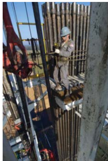
A derrick man works pipe stands from the monkey board of Grey Wolf Rig 103, Angelina, Tex. (Fig. 1; photo from Grey Wolf Drilling Co. LP).
